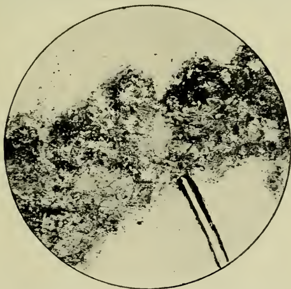
Fig. 3.—Photomicrograph of darkened spot near center of head of rail. Transverse section, 100 diameters magnification
